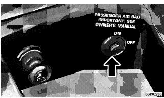
Passenger Airbag ON/OFF Switch
